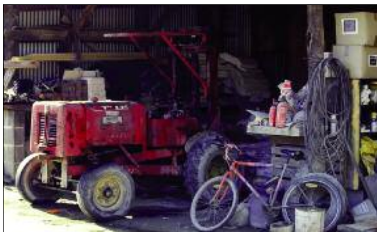
The electrical, fuel, and exhaust systems of tractors and other vehicles parked near barns can cause fires—and the vehicles and clutter around them can impede firefighters' access.
